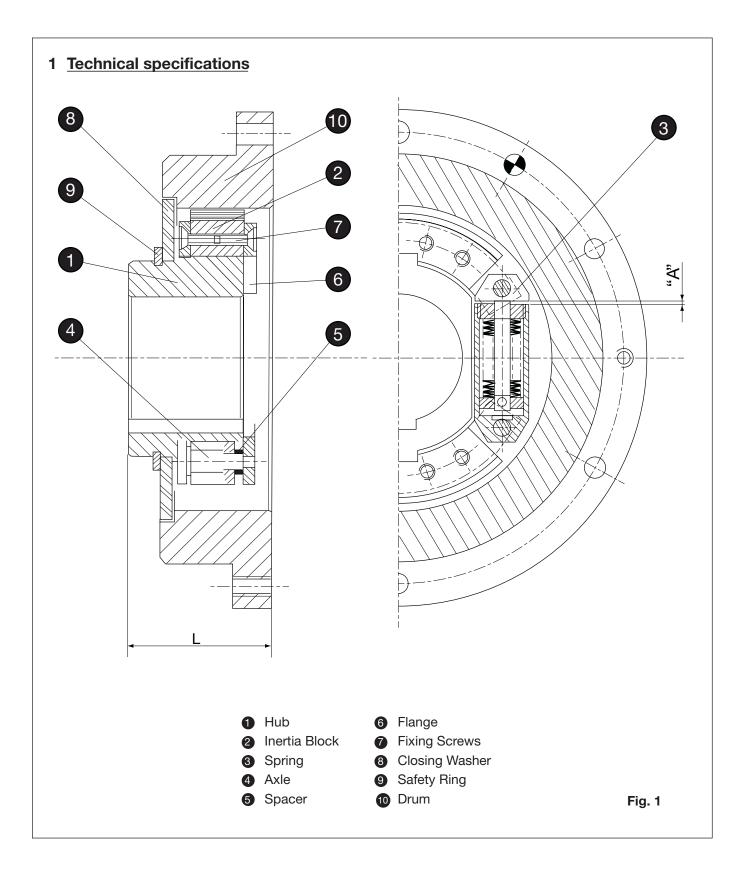
The FC-G - C140 centrifugal brake is a device operating with delayed actuation that is to say, the pressure between the friction surfaces is achieved by the centrifugal force resulting from the rotation of the driving input. The engagement or disengagement is therefore driven only by action upon the input side.
