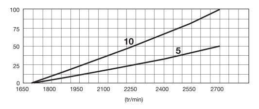
Nil torque (RPM) 1850 Nominal torque (RPM) 2800
