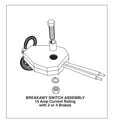
Activated only in the event of a trailer breakaway emergency, the breakaway switch remotely activates the independent safety circuit of the trailer brake systems. Sonic welded case protects electrical component against water and sun.
