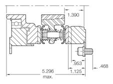
Outside Mounted Flush Backing Plate
