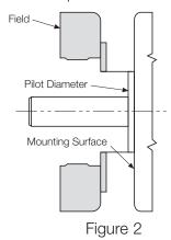
magnet mounting flange (refer to illustration drawings page 38 & 42) to aid in the proper positioning of the magnet.
