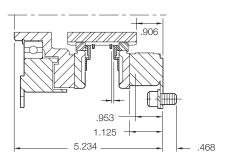
Outside Mounted Flush Backing Plate
