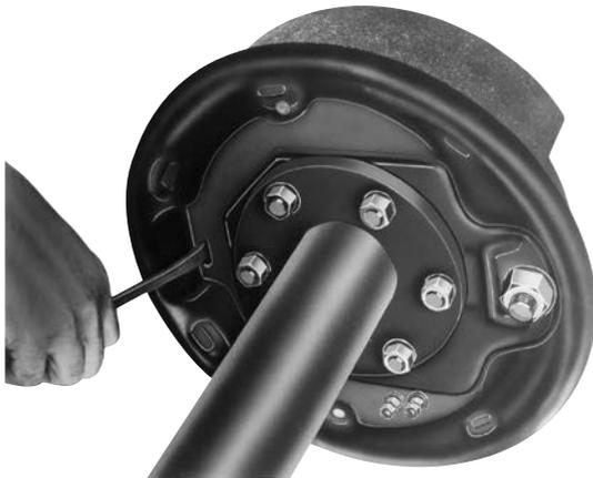
**Figure 4 - Brake Adjustment**
