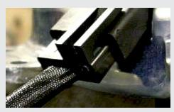
Low profile connector allows for easy replacement of cable assembly.
