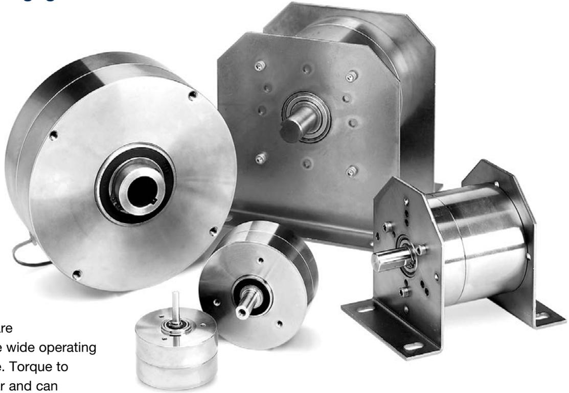
Warner Electric Precision Tork magnetic particle clutches and brakes are unique because of the wide operating torque range available. Torque to current is almost linear and can be controlled very accurately. The unique features of the magnetic particle clutches and brakes make them ideal for tension control, load simulation, cycling/indexing, and soft starts and stops.
