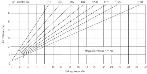
Maximum Braking Force = 36kN
