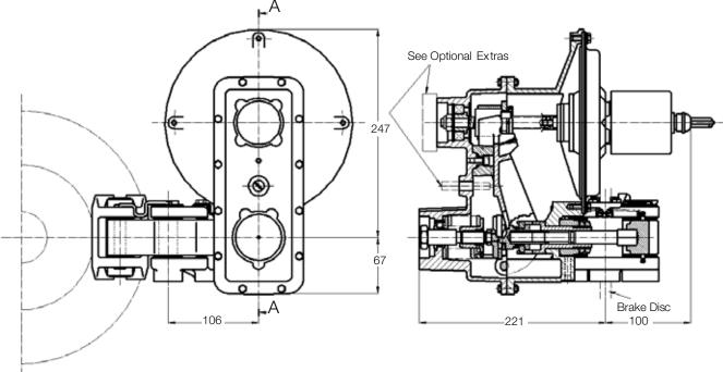
3 off Caliper mounting bolts M12 grade 8.8 and nuts grade 8, tightening torque 80 Nm - Not supplied with caliper
