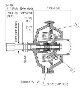
Measurements in metric, inches in brackets
