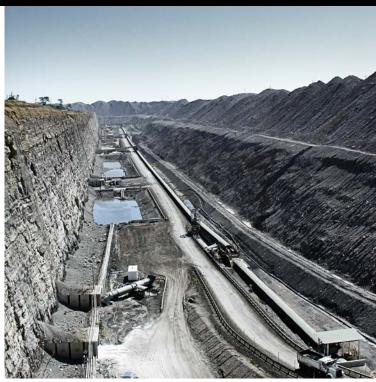
Conveyors are efficient in industrial mines and metallurgical plants. But like other heavy equipment, they pose hazards to employees and to the safety of the equipment, as the operation is mostly unmanned due to its distance, terrain and profile. Therefore, it is imperative to develop an intelligent soft braking system to address the starting and stopping requirements under various load conditions.
