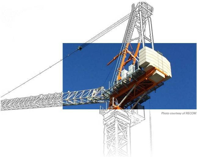
**Luffing tower cranes** are used in building projects where space is limited. A luffing crane can raises or lowers its boom while the hook is positioned on the proper location. Moving the boom pulls the hook up and down or inwards and outwards.
