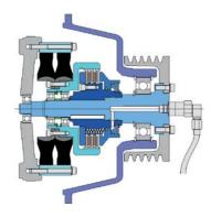
Stromag KHA with flexible Periflex®VN couplings for drives particularly subject to torsional vibrations. Connection for SAE flywheels.
