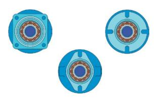
Connection flanges according to SAE standard or customer specifications.
