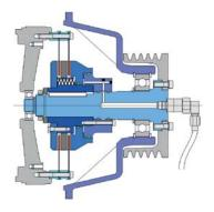
**Stromag KHM** for engine mounting. Backlash-free power transmission via diaphragm guided pistons and friction linings. Drag torque free when open.
