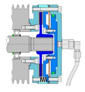
**Stromag KHM** as a shaft-pulley connection. Backlash-free power transmission on pulley side through external body and piston with diaphragm guidance.
