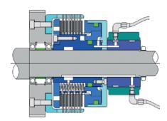
**Stromag KMK** for use in gearboxes (wet operation) with optional disc oil flushing.
