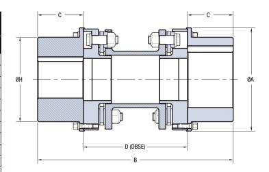
\* For Large Hub H = A. \*\* The inclusion of additional features such as packing rings, shims and/or electrical insulation will increase the D min. (DBSE: Distance Between Shaft Ends) and B min. dimensions.
