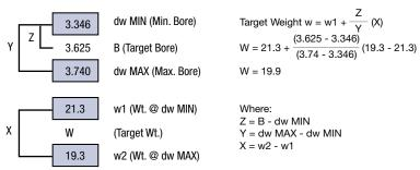
Note that the same method can be used to determine actual Torsiloc transmissible torque ratings for bores that are in between the min and max.
