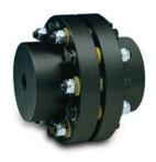
The E-flex pin and bush couplings accept parallel, angular and axial misalignment and can provide considerable torsional flexibility.
