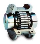
State-of-the-art design from Bibby Transmissions, the original grid coupling manufacturer. 54 Series/Bibby 2000 Series is an all-metal coupling that provides positive protection against the damaging effects of shock loads and vibration. Both horizontal cover (H), and vertical cover (V) designs are available. Grid couplings are an excellent choice where torsional flexibility/ vibration damping are primary concerns.
