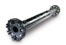
These floating shaft couplings are specifically designed for long span applications. Incorporating composite tubes, which can be specified for spans of 10+ meters, they weigh up to 80% less than steel and eliminate the cost of bearing supports and other structures.
