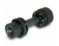
Torsiflex couplings are specifically designed for the process pump and general industrial markets. Torsiflex is an all-metal disc coupling requiring no lubrication which incorporates a plug-in feature to allow installation and removal without disturbing the pump alignment. Standard units are compliant with API 610 (American Petroleum Institute) and the more demanding API 671 standard can be achieved. In addition, the coupling is certified to meet ATEX 2014/34/EU.
