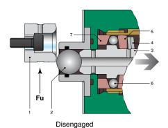
A suitable switch can be incorporated in the assembly to switch off the drive motor or operate a warning device when the Torque Limiting assembly disengages. After first ensuring that the drive is isolated, resetting is a simple matter of first realigning the flanges and then tapping each module plunger back with a soft mallet to allow the circle of balls to return to their original position and the large steel ball to return to its location in the detent pocket.
